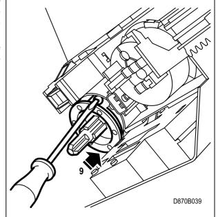
13 Position the control panel and fit the telescoping control shaft.
